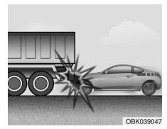
• Frontal airbags may not inflate in "under-ride" collisions where the collision energy is absorbed above the vehicle's front bumper.
