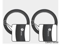
Your vehicle is equipped with asymmetric tires, when you replace the tires, check the inside and outside of the tire.
