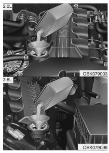
If it is near or at L, add enough oil to bring the level to F. **Do not overfill.**
