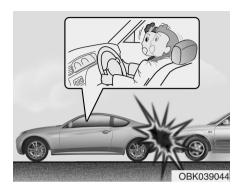
Frontal air bags are not designed to inflate in rear collisions, because occupants are moved backward by the force of the impact. In this case, inflated air bags would not to provide additional occupant protection.
