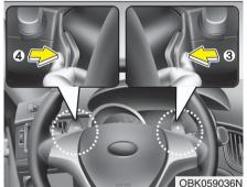
In sport mode, it is possible to shift the gear by using either the shift lever or the steering wheel shift paddles (dynamic shift).
