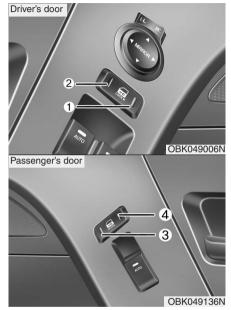
D050202ABK-EU **With central door lock switch**Operate by depressing the central door lock switch.
