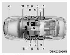
The SRSCM continually monitors all SRS components while the ignition switch is ON to determine if a crash impact is severe enough to require air bag deployment or pre-tensioner seat belt deployment.
