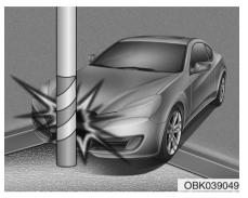
· Air bags may not inflate if the vehicle collides with objects such as a utility pole or tree, where the point of impact is concentrated and the collision energy is absorbed by the vehicle structure. C041100ABH
