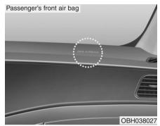
The purpose of the SRS is to provide the vehicle's driver and/or the front passenger with additional protection than that offered by the seat belt system alone in case of a frontal impact of sufficient severity. The SRS uses sensors to gather information about the impact severity.
