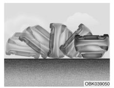
· Side impact and curtain air bags may not inflate in rollover accidents. Unless the side of the vehicles is struck with sufficient force to cause airbag inflation to occur.
